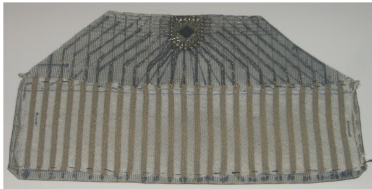
Figure 3.3: The first version—A PCB with an Atmega is connected with the pinstripe textile with conductive thread.
