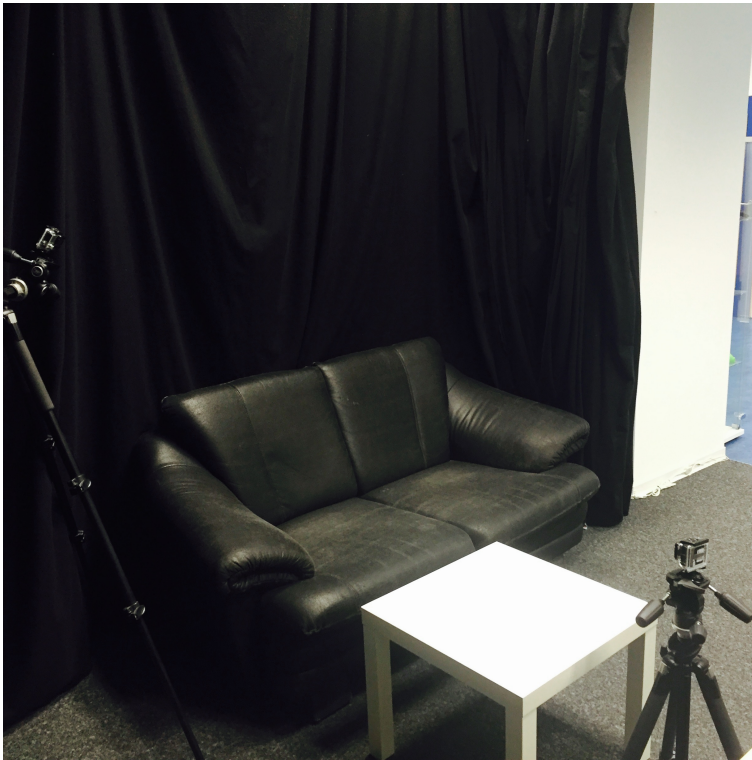
Figure 4.1: The study setup for the exploratory study. We simulated a part of a living room environment with a couch, a coffee table, and a curtain at arms length of the user. The gestures were recorded using two GoPro™ cameras.
