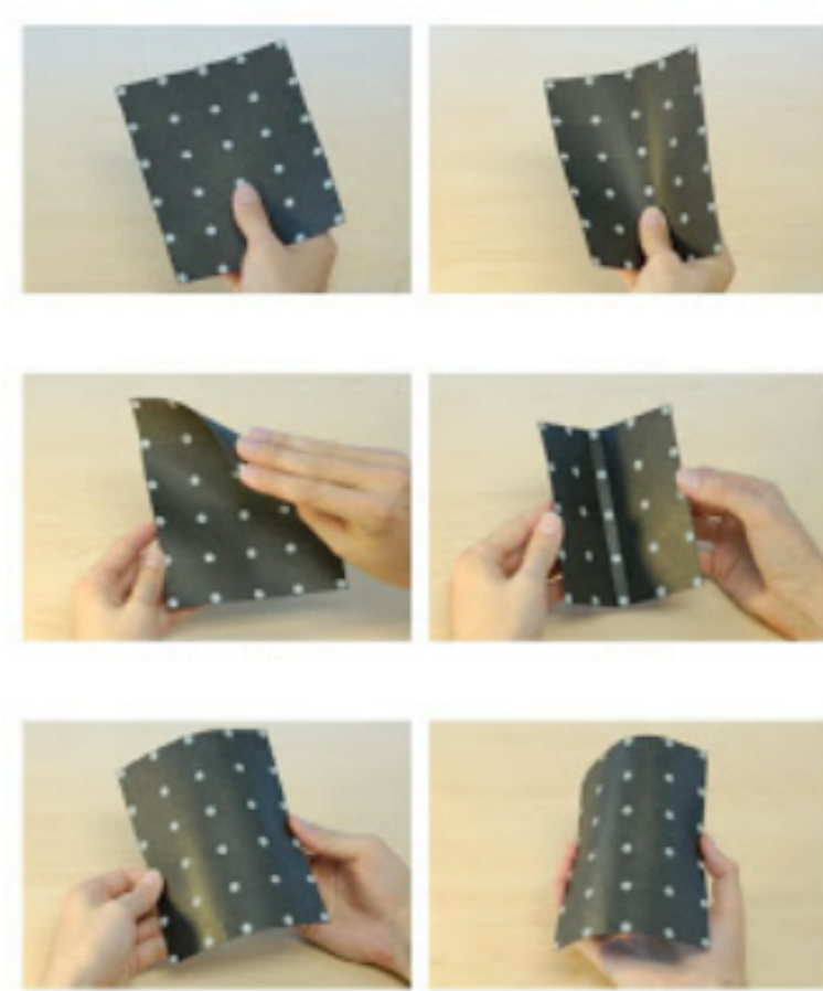
Figure 2.9: The supported deformation interactions of the FID device include thumb slide, scoop, top corner bend, fold, leafing, and squeeze.
