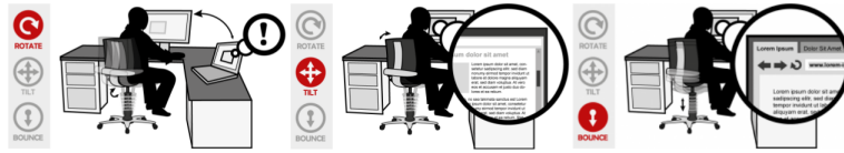
Figure 2.5: The interactions possible with the chair as an ubiquitous computing device: rotate, tilt, bounce up and down.
