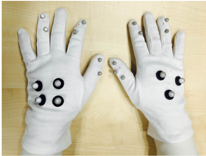
Figure 6.3: Gloves used for the study with ten markers on each hand. The marker layout was varied to aid during the manual gap filling post study.
