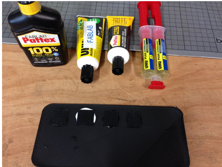
Figure 3.21: Velcro-PLA adherence test
