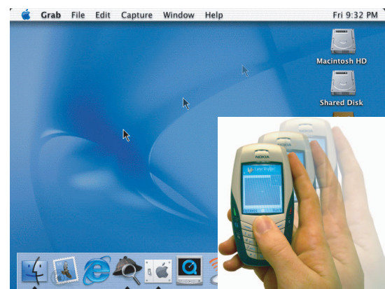
Figure 5. The Sweep technique uses camera input and optical flow image processing to control a cursor.
