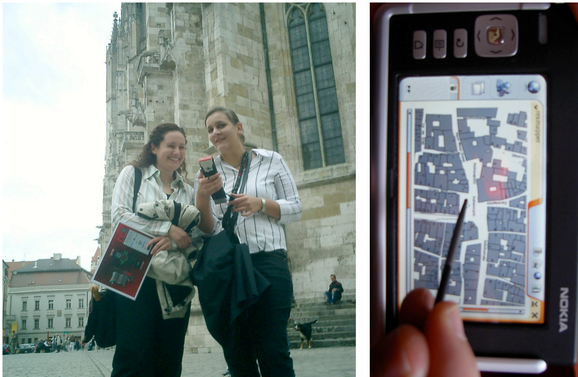
Figure 5.14: For the playability tests, Wizard of Oz techniques were applied using the Nokia 770 tablet. A test administrator uses the tablet to manually input the players' position as they follow the players through the city to simulate a fully functional location detection system.
