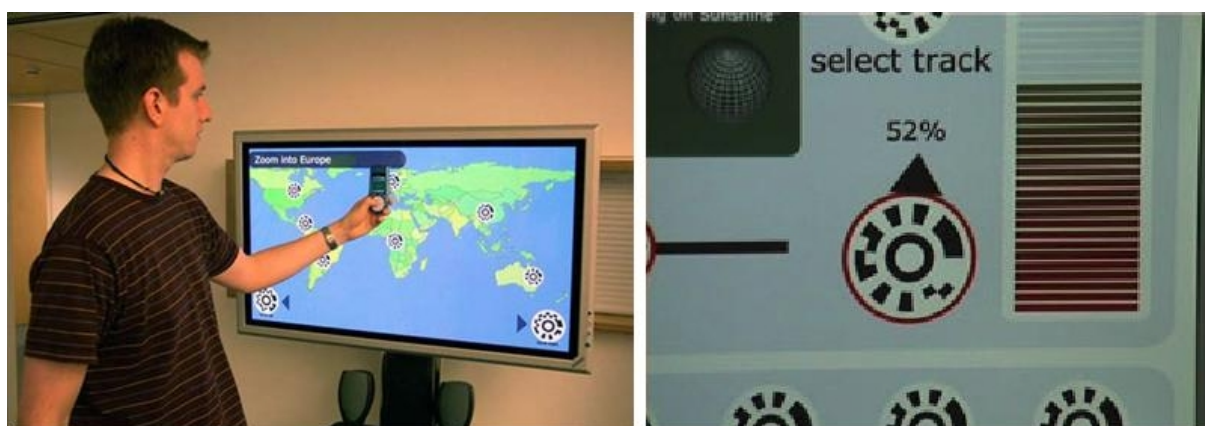
Figure 2.5: Using the phone to manipulate tagged widgets such as buttons, dials, and sliders (Madhavapeddy et al. , 2004).
