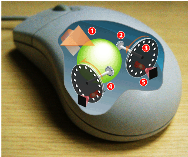
Figure 4.3: An optical-mechanical mouse: (1) Motion across the desktop surface moves the ball. (2) Grips transfer the ball movement to turn (3) optical encoding disks. (4) Infrared LEDs shine through the holes. (5) Infrared sensors accumulate light pulses and convert them into motion along the X and Y axes. (Source: Wikipedia)
