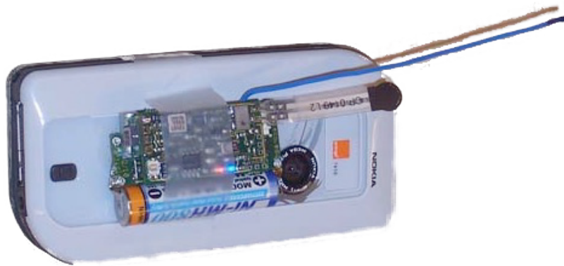
Figure 3.27: Back view of a mobile phone augmented with a Smart-Its sensor board in iStuff Mobile. The sensors can be attached to the phone in whatever position the designer finds most appropriate. The pictured Smart-It contains a 3D accelerometer, microphone, and sensors for light, pressure, temperature, and voltage.
