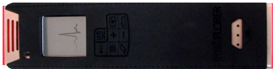
Figure 5.2: The REXPLORER “detector” consists of a Nokia N70 mobile phone and a GPS receiver packaged together in a protective shell. A soft and stretchable textile overlay with a zipper on the back transforms the standard phone keypad into an 8-key game interface.
