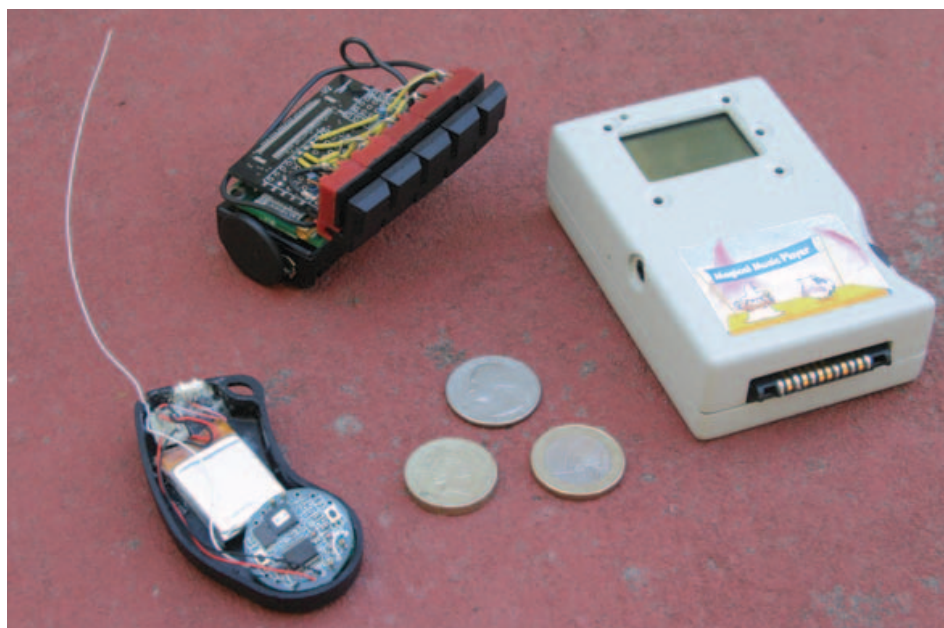
Figure 3.26: Hardware prototype components, including tagged presentation remote control (upper left), prototype mobile device (right), and RFID reader (bottom left). The remote control is tagged with an RFID tag (black circle on end), and the RFID reader is exposed to show its inner circuitry. (A Euro, a British Pound, and a U.S. quarter are included for scale.)
