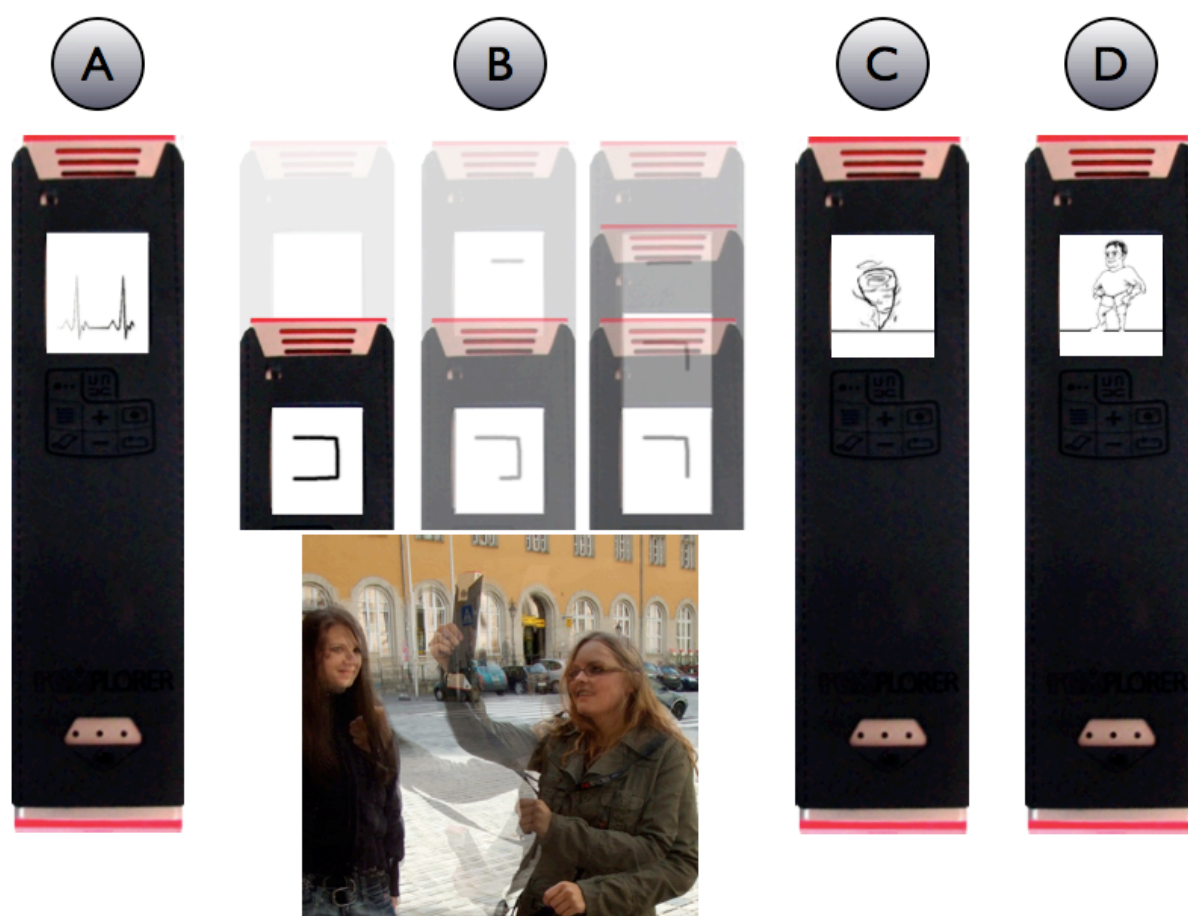
Figure 5.6: (A) The excited heartbeat indicates that the player is in a hotzone and can interact with a spirit. (B) The player casts a spell by drawing one of the gravestone symbols in the air. Audio feedback, as well as visual feedback is given to the player displaying the gesture progress. (C) An element animation (in this case ‘wind’) confirms which gesture was recognized, whilst the attached audio plays back. (D) The likeness of the character is displayed on the screen as the spirit communicates with the player.
