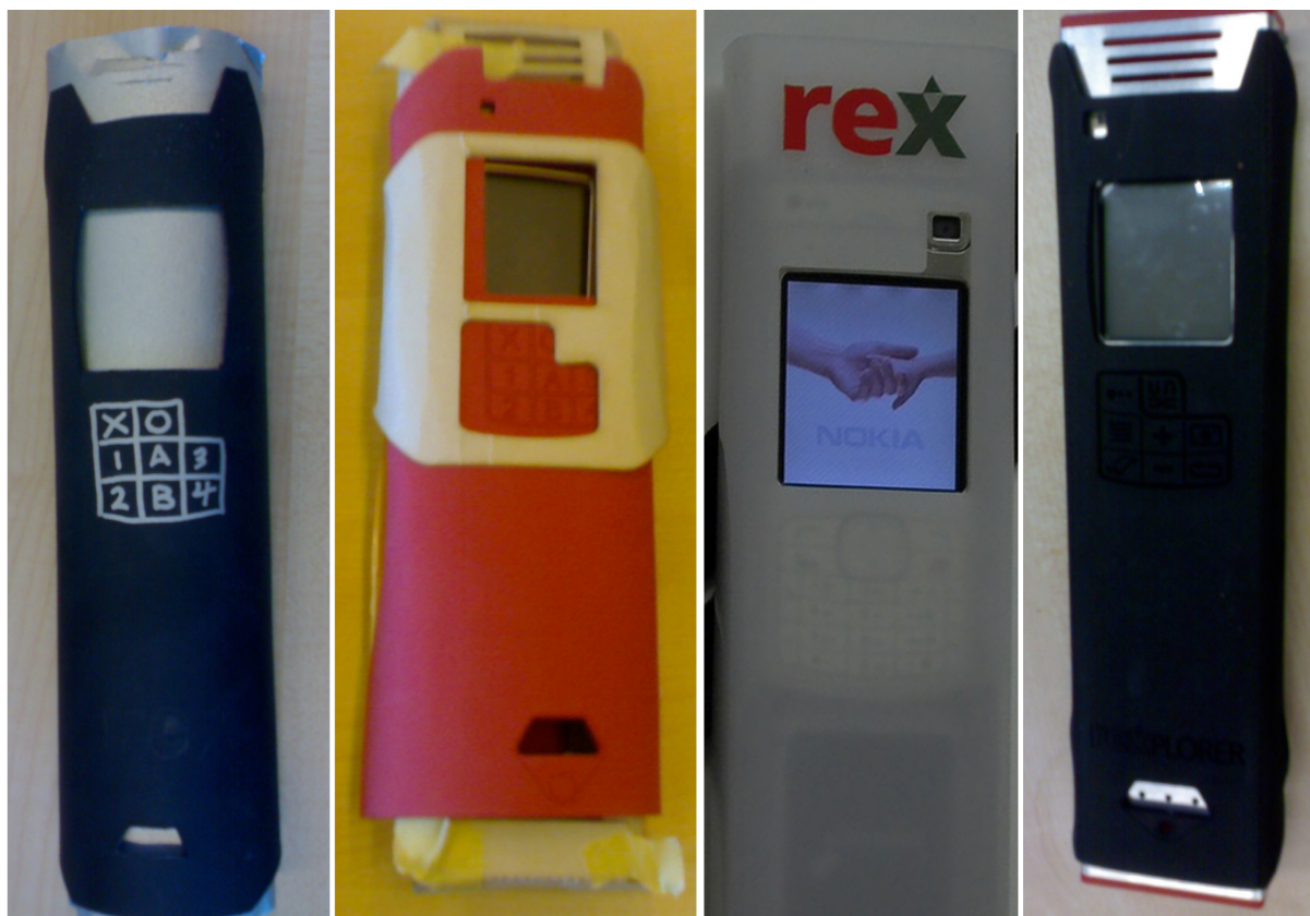
Figure 5.13: The detector houses the GPS receiver and the mobile phone in a protective shell; it is wrapped by a stretchable and soft textile with custom key labels. (Left) An early prototype consisting of construction paper, wrapping a wooden core, and buttons sketched on with a metallic pen. (Middle-Left) A more advanced prototype consisting of cardboard, a real mobile phone, and a close to final textile skin. (Middle-Right) A prototype for materials exploration, this plastic design housed both the mobile phone and the GPS device, but did not properly expose the buttons. (Right) The final design with an aluminum protective shell covered in a soft textile wrapping.
