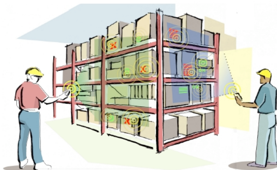
Figure 2.9: A warehouse scenario employing RFIG. The users can highlight and select objects of interest combining a handheld projector and embedded light sensitive RFID tags (Raskar et al. , 2004).
