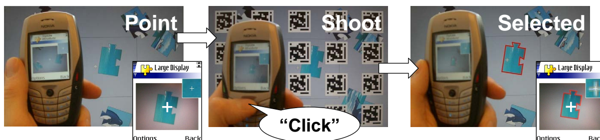
Figure 2.8: Point & Shoot technique: (Left) The phone display is used to aim at a puzzle piece on a large display. (Middle) Pressing the joystick indicates selection and a visual code grid flashes on the large display to compute the target coordinates. (Right) The grid disappears and the targeted piece highlights to indicate successful selection. (Ballagas et al. , 2005)
