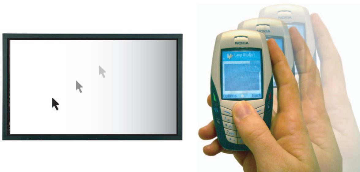
Figure 2.4: The Sweep technique uses camera input and optical flow image processing to control a cursor (Ballagas et al. , 2005).
