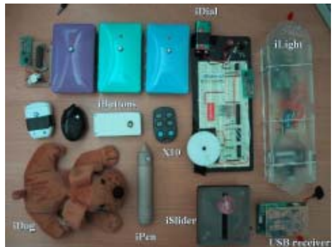
Figure 3. Various iStuff. The iDog sends a button press event when turned over. The iPen is an augmented SMART board pen, where the embedded button operates as a "right click" to the Windows OS. The X10 buttons are standard X10 hardware. All other devices work through a simple RF receiver that plugs into the USB port of the Proxy PC.
