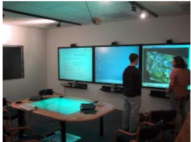
Figure 1. The interactive room (iRoom), showing its three SMART boards, interactive table, wireless keyboard and mouse, an other wireless input. The unlit screen on the left is part of the high-resolution, interactive "mural" [Mural01]
