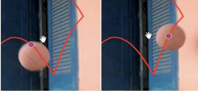
Figure 4.5: Problem when using shortest distance. A very small mouse movement causes a huge leap in the playback. This disturbs the natural mapping between input and output motion, and surprises users.
