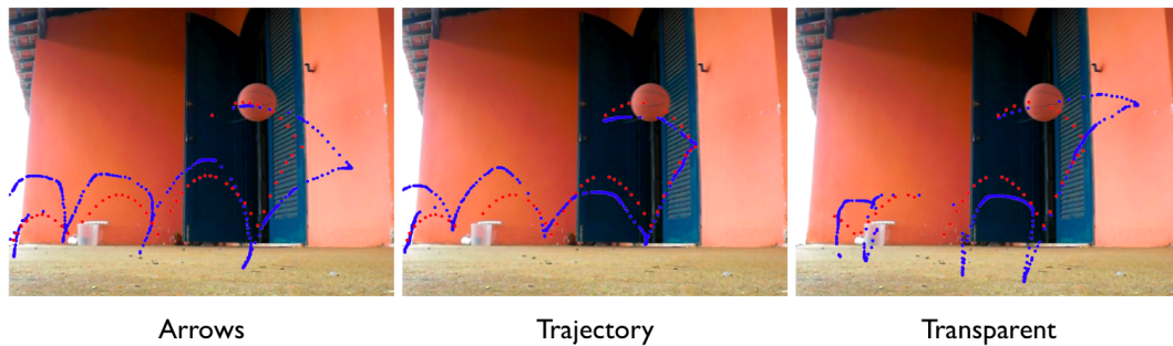
Figure 4.4: Mouse (blue) and corresponding object (red) motion with three different visualisations. For wave-like trajectories, the spatio-temporal approach to calculate the next frame frequently leads to jumps in the video playback during drag interactions. Hiding trajectories increases the level of difficulty while full trajectories allow for high accuracy.
