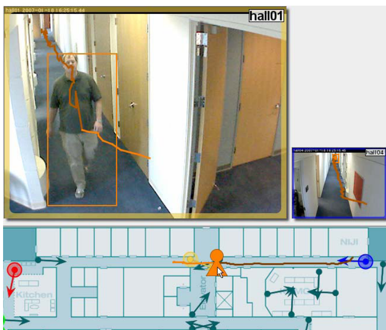
Figure 2.7: Trailblazing (by Kimber et al. [2-5 July 2007]) Viewer showing trails in video and floor plan view. The user may scrub video by dragging a person along their path in the video window or on the floor plan.
