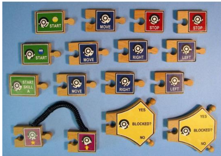
Figure 2.5: Tern blocks used to create a chain of commands for a robot ([Horn and Jacob, 2007]).
