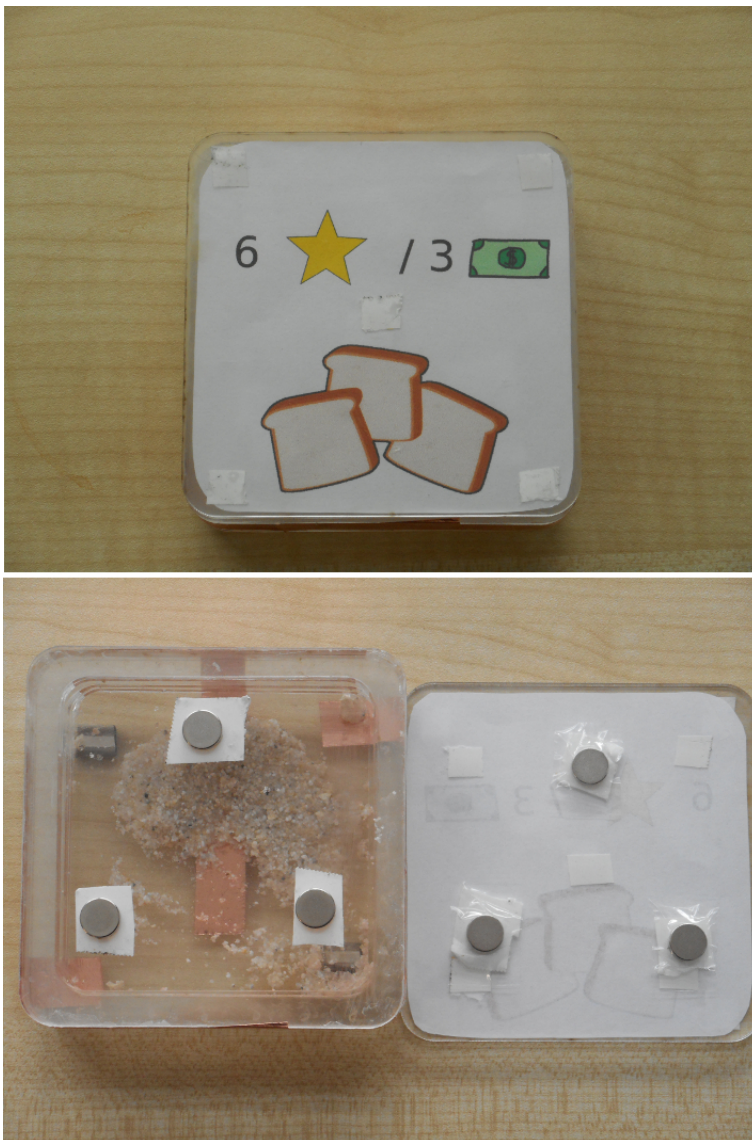
Figure 3.8: Toast tangible with its cover attached and with its cover detached, showing the magnets.
