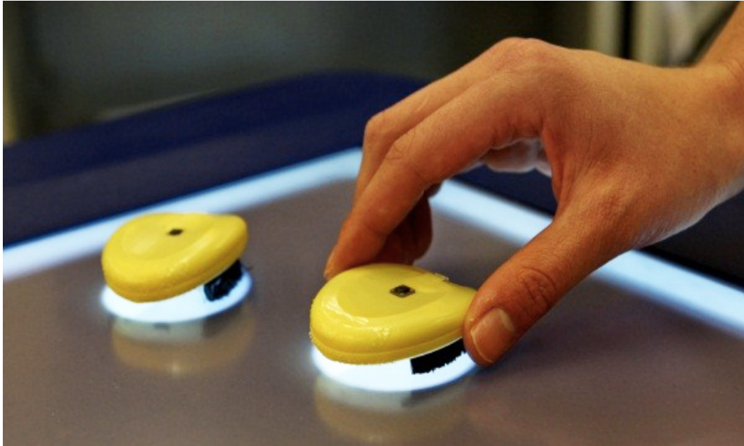
Figure 2.10: TouchBugs are built upon small brushes on which they move, controlled by vibration patterns. Image taken from Nowacka et al. [2013]
