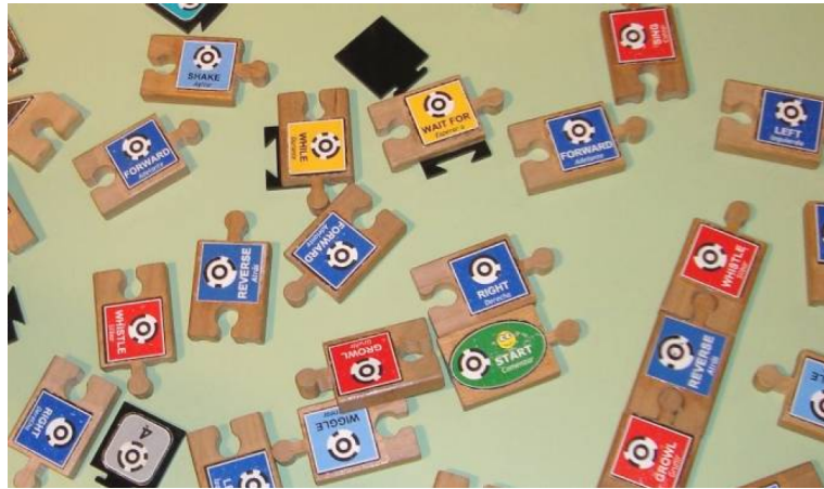
Figure 2.4: Tangible programming blocks as used in Tern. They are shaped like puzzle pieces and connect to each other to form a chain.
