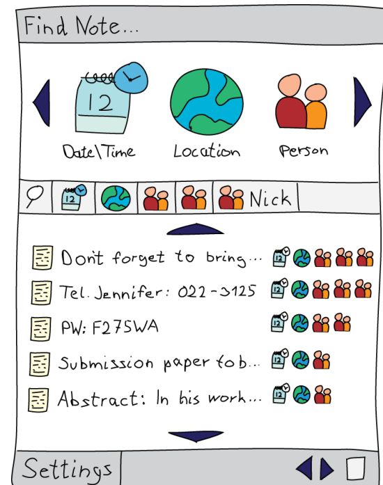
Figure 2: Paper prototype of the note retrieval screen. The association bar shows the available types. Dragging items to the search bar below automatically updates the search results. Space is conserved by minimizing previous items, which can be reopened. Removing an item is simply done by dragging off the bar. Below it the search results are shown. The icons next to each result indicate its rating: for each search hit the corresponding icon is displayed.
