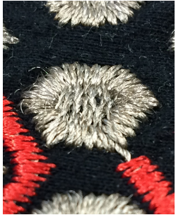
Figure 2: The conductive pads are embroidered in a circular manner, such that movement is not restricted by threads snagging onto each other.
