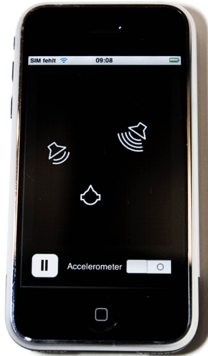
Figure 3.13: Simple OpenAL Demo Application Running on the iPhone: the listener and the sound sources can be moved around and the rendering engine adapts the audio stream accordingly.
