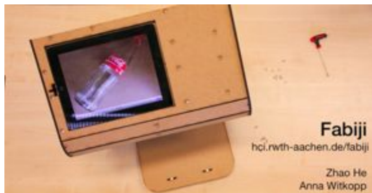
Figure 2.3: The Fabiji prototype. An iPad enclosed in a kiosk-stand cut out of medium-density fibreboard with a laser cutter
