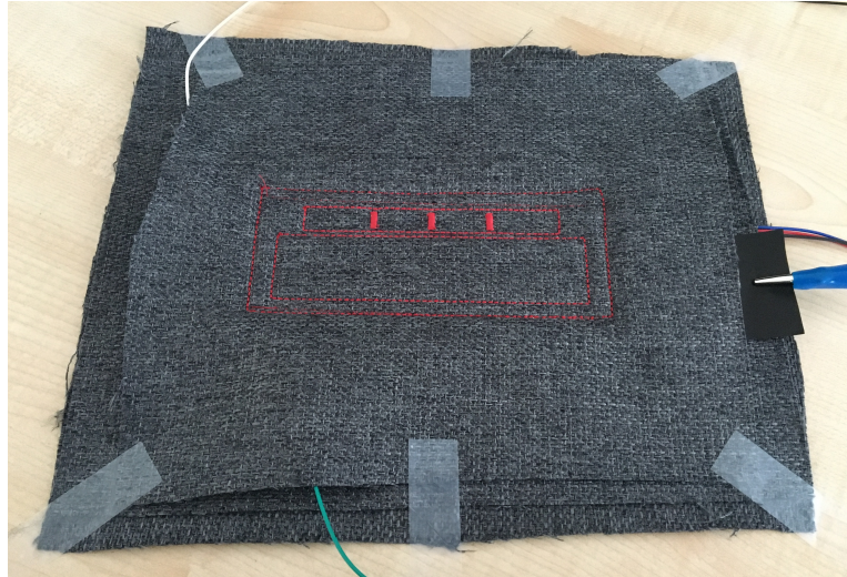
Figure 3.9: Figure of prototype 2. Here again, the slider is realized by the inner, narrow rectangle with the three-tick-mark design. Below the slider, a pressure sensitive area is located that is marked by the wider rectangle.
