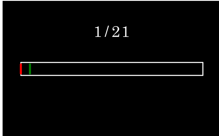
Figure 4.2: The visualization of the user input versus the expected input. The red line indicates the current user input and the green line corresponds to the target value that needs to be set. The counter above indicates how many of the 21 target values were already reached.
