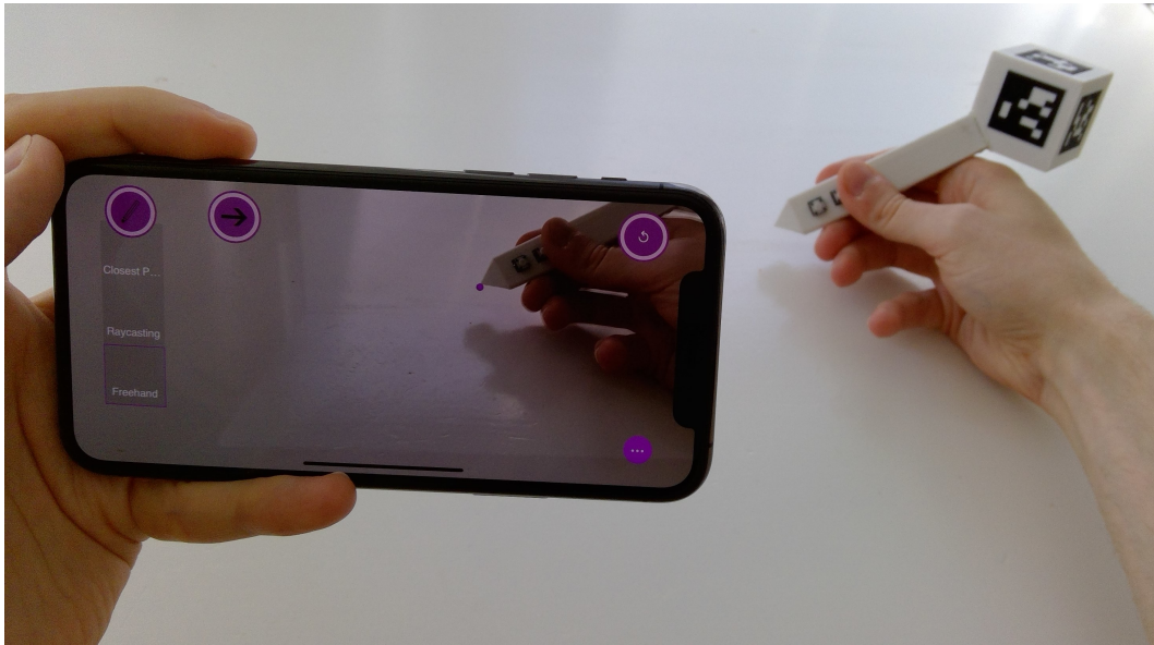
Figure 2.3: The ARPen system in use. The marker box at the end of the pen needs to be in the camera frame to be tracked correctly.
