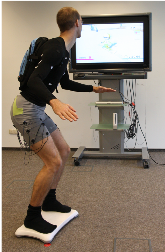
Figure 6.2: Experimental setup: While playing a snowboarding game on the Wii Fit console the test person had to recognize the perceived feedback patterns (belonging to categories C1 and C2).
