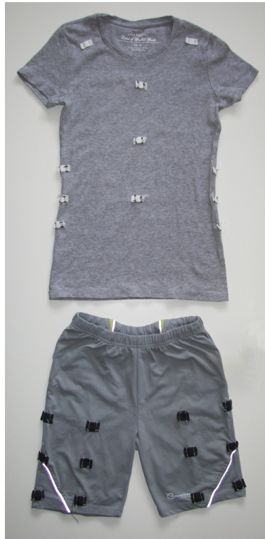
Figure 5.8: The clothes used during the study, motors were inserted inside the small pouches.
