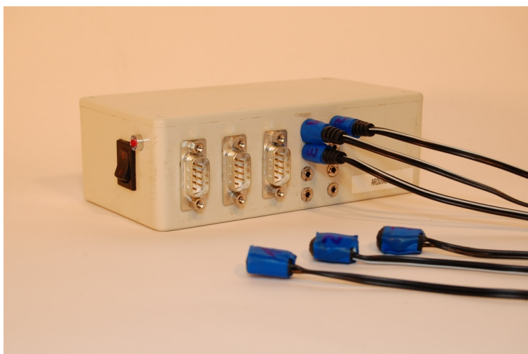
Figure 4.2: SensAct Box: The main part of the hardware platform we used for our user studies, showing the SensAct box and three actuators.
