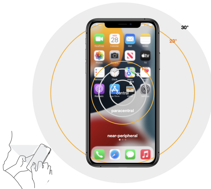
Figure 3.1: An example of the visual angle on the mobile screen(iPhone XS): the visual field covers the entire area of the screen within the near-peripheral vision.
