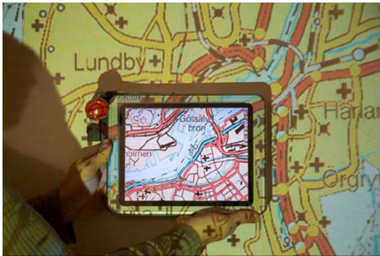
Figure 1.1: Sanneblad06: A user holds up a tablet PC in front of a large projected image to view details
