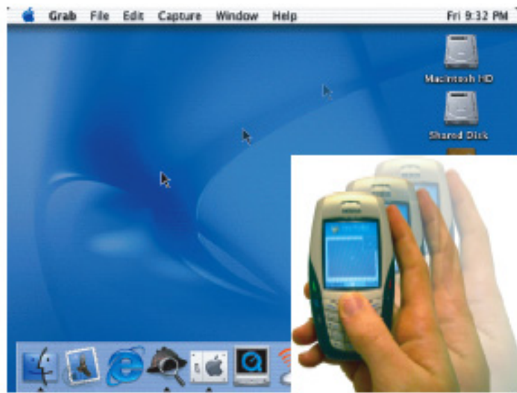
Figure 1.2: The sweep technique can be used to control a cursor on the large public display like an optical mouse
