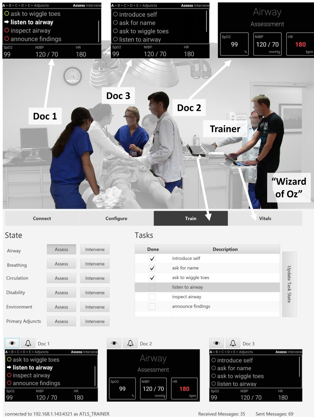
Figure 5.1: Experimental setup for simulation A. The three highlighted trainees are wearing Google Glass. By using a tablet application, the trainer administered the checklist remotely and the "Wizard of Oz" updated the vital signs manually.
