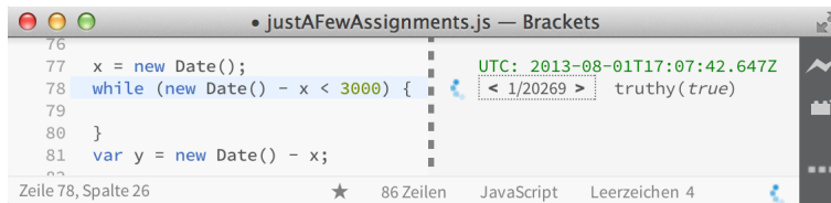
Figure 4.11: Long-running code that is currently being executed. A spinning indicator in the lower right corner of the window shows the current execution and another spinning indicator in line 78 shows that this is the last line that was executed so far.
