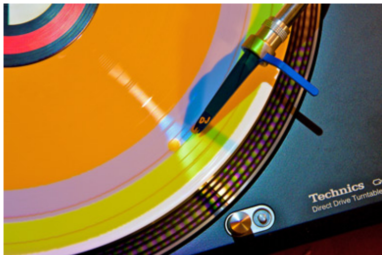
Figure 3.7: The augmented interface DiskPlay. Next to the tonearm is a cue point which spins on its orbit, denoted through a black circle.
