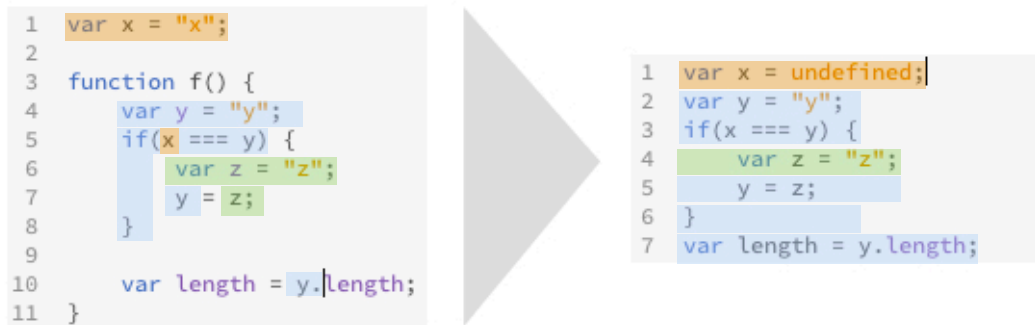
Figure 4.3: Building the context (right) for line 10: Fiddlets looks for lines that reference y (blue). Since line 7 references y , but also references z , Fiddlets includes lines referencing z (green). Since the variable x is declared outside of the scope of function f , x is considered undefined (orange).
