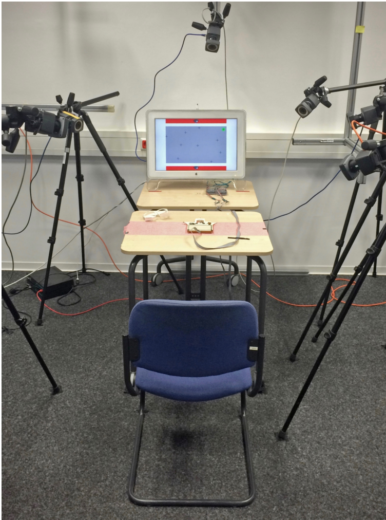
Figure 5.2: Participants were seated in front of a 73.5cm high and 70.0cm wide measurement table, being away 100cm from the distant screen (height: 31.5cm, width: 50cm). To avoid participants from stabilizing throughout the study, we decided to choose a chair (length: 44cm, width: 43.5cm, height: 55cm) without arm rest.
