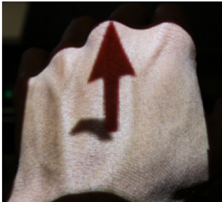
Figure 2.9: 3D arrow to guide user's movement in Light-Guide (Sodhi et al. [2012])
