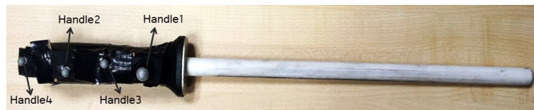
Figure 4.3: Reflective markers placed on the handle of the honing rod
