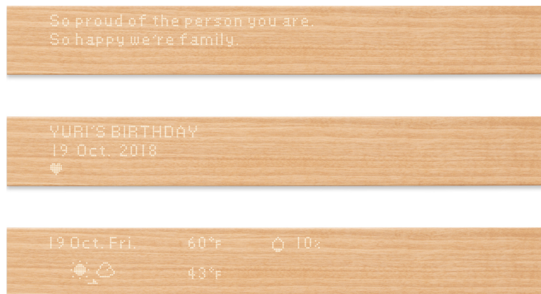
Figure 4.6: The smart home management hub Mui : Smart devices may be connected to the interface through an application, and messages, calendar events, and weather forecasts, as well as household appliances such as lighting, can be shown and managed. Image taken from Oki [2016].
