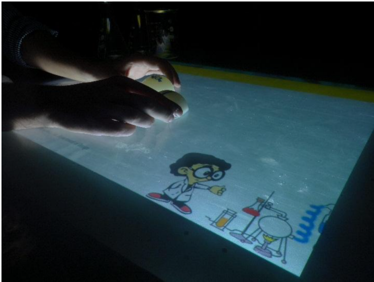
Figure 4.5: ChemicAble prototype: 20 Hemispherical tokens were used to represent the first 20 elements of the periodic table. When an atom token is put on top of the table, its valence shell is displayed surrounding the token. Image taken from Agrawal et al. [2013].
