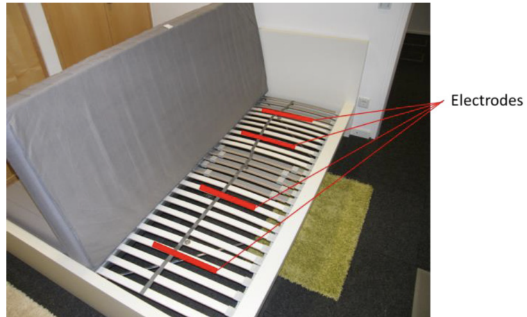
Figure 3.5: MoviBed prototype: sensors are mounted to the bed frame in order to assess the user's movement while sleeping. Image taken from Djakow et al. [2014].
