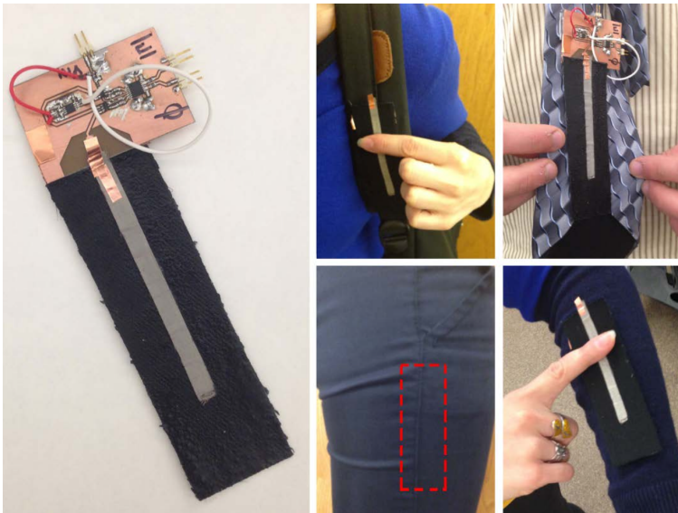
Figure 5.5: SwitchBack may be used to a variety of items to make them interactive. For example, on a backpack, on tie, beneath the pant leg and on a sleeve. Image taken from Hughes et al. [2014].
