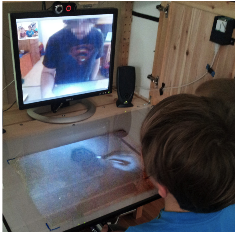
Figure 4.1: The ShareTable prototype being used by a Parent and child at home: the display shows the distant parent, while the local table surface shows a projected picture of the parent's table surface, where he is sketching. Image taken from Yarosh et al. [2013]
