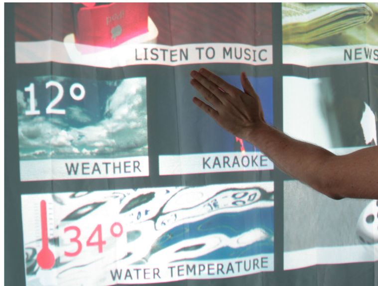
Figure 3.1: The interactive shower curtain: information is projected on the shower curtain, which may be manipulated by touch. Image taken from Funk et al. [2015].
