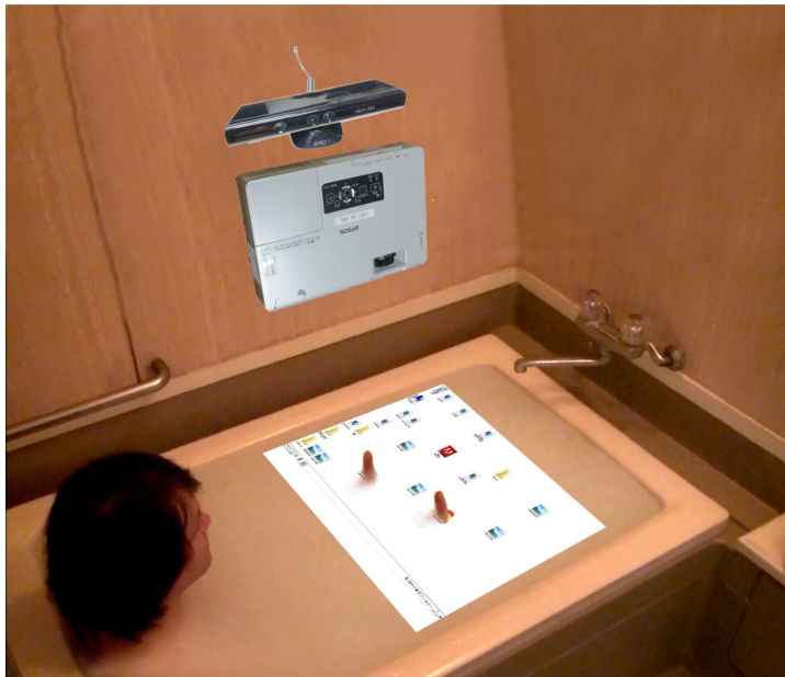
Figure 3.3: Aquatop's application scenario: information is projected on cloudy water surface, and poking is the modality that is used here. Image taken from Koike et al. [2013].
