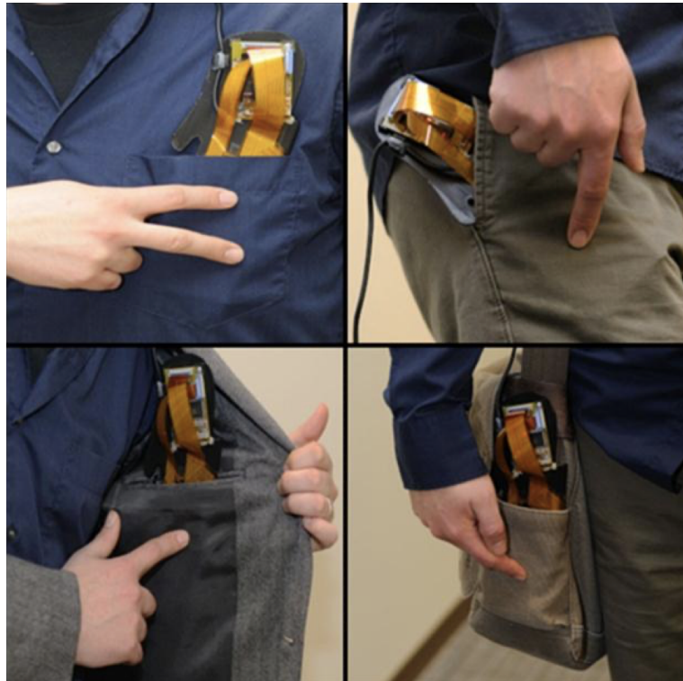
Figure 5.2: Touching or brushing the interface’s surface interacts with the PocketTouch interface, a capacitive sensing prototype. Image taken from Saponas et al. [2011].
