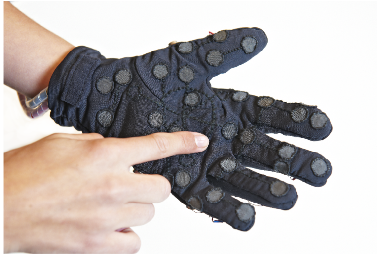
Figure 4.2: The Lorm Glove's input surface: The left hand may wear the Lorm Glove , while the right hand can tap the buttons that depict the letters. Messages may also be received on the phone and translated for the user into Lorm alphabet via micro vibration motors. Image taken from Gollner et al. [2012].
