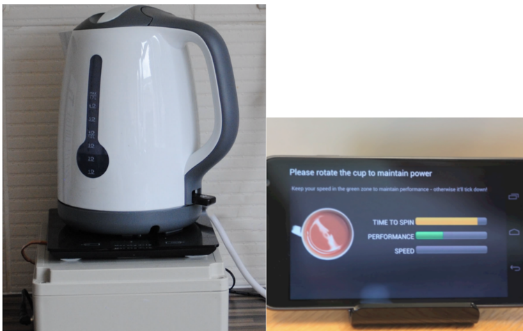
Figure 5.10: The Stropky Kettle prototype and the punishment system on a mobile device used to punish the users, when they overflow the kettle Image taken from Cowan et al. [2013].
