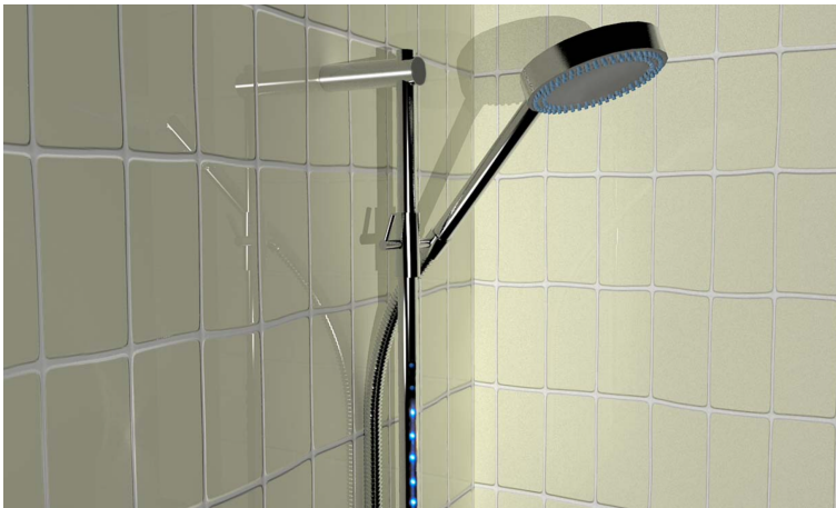
Figure 5.9: An example of the Show-Me interface in use in the shower: the LEDs are built right into the shower's sliding bar, putting them right in the user's line of sight. One LED light represents 5 liters of water used. Image taken from Kappel and Grechenig [2009].
