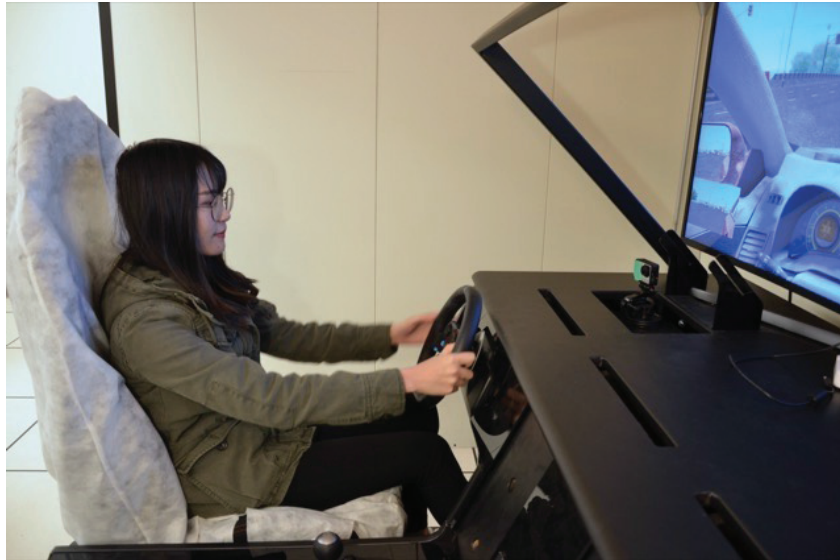
Fig. 1. A participant performing slow breathing exercises in the simulated driving setup. A customized haptic seat made of a grid of vibrotactile motors guides her breathing.
