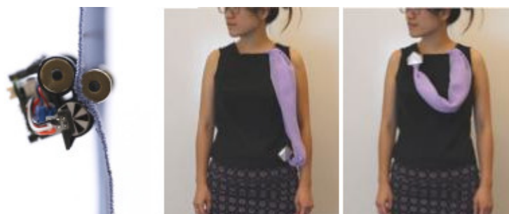
Figure 2.8: Left: Rovable is attached to fabric through magnetic mechanisms. Center-Right: Rovable pulls at a scarf and wraps it round the wearer depending on ambient temperature. Dementyev et al. [2016].
