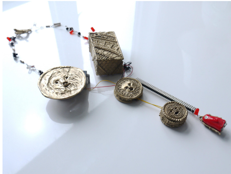
Figure 2.10: A large jewelry piece with rotating (via motor) and flashing (via LED) components. Ju [2016].
