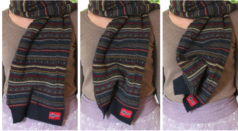
Figure 2.7: Scarfy. Self-actuating scarf by using SMAs. von Radziewsky et al. [2015].
