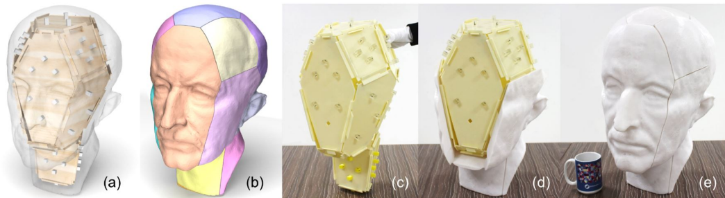
Figure 2.8: In the CofiFab process the core is assembled from milled parts and the outer shell is assembled from printed parts, to increase speed while keeping detail. Image adapted from Song et al. [2016].
