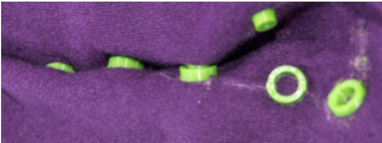
Figure 2.10: 3D printed fabric connectors. Image adapted from Rivera et al. [2017].
