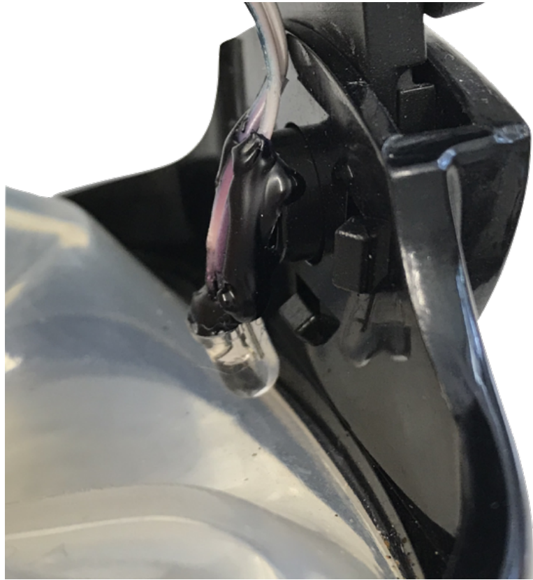
Figure 3.1: LED insulated and attached between the silicone and frame of the diving goggles using hotglue.
