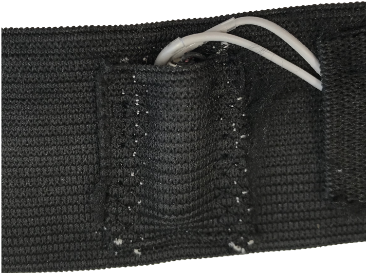
Figure 3.4: Piece of the stretchband sewn to the headband as a bag for the vibration motor.
