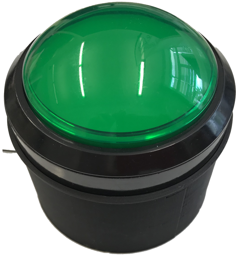
Figure 3.6: The botton and the 3D printed case. To be pressed by the user when he recognizes feedback.
