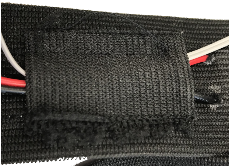
Figure 3.5: Pieces of the stretchband sewn to the headband as wireway for better cable management.
