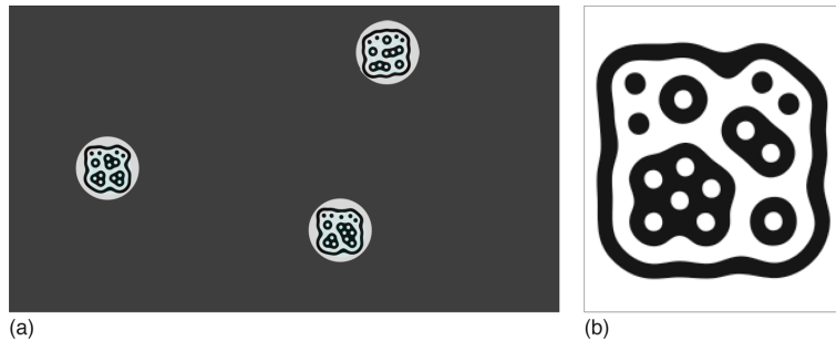
Figure 4.5: Tracking with the reacTIVision framework. (a) Camera view. (b) A fiducial marker
