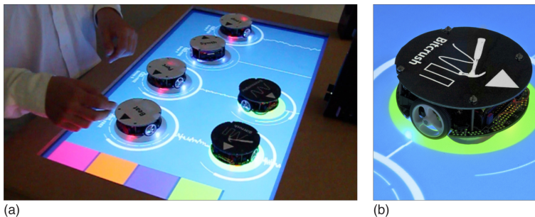
Figure 1.2: Musical instrument with Tangible Bots. (a) The user interface of the musical instrument. (b) A Tangible Bot. (All figures from [Pedersen and Hornbaek, 2011])
