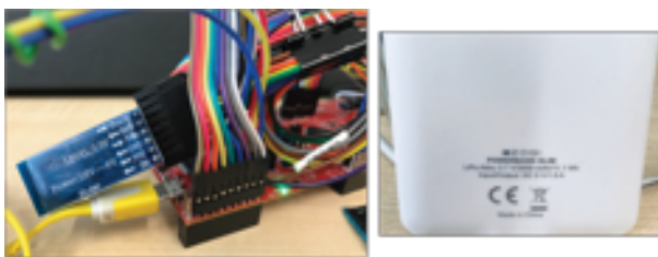
Figure 4.9: Left: picture of the Bluetooth module connected to the microcontroller. Right: backside picture of the power bank we used for our prototype, technical specifications are visible.
