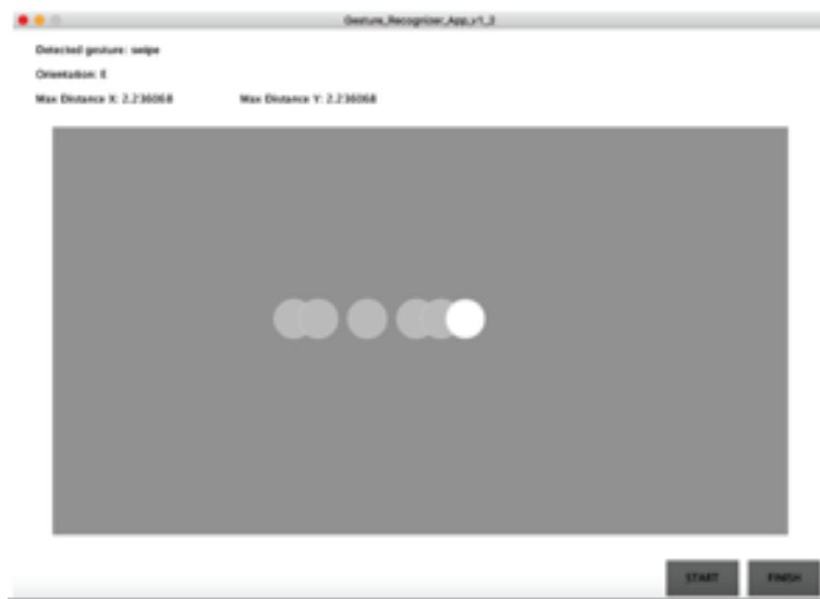
Figure 4.8: Screen of the Gesture Recognizer App working. We observe the detection of a gesture and how the user's finger is drawn following the motion of the gesture. The app prints the detected gesture, the orientation and the x and y axis length the gesture followed.
