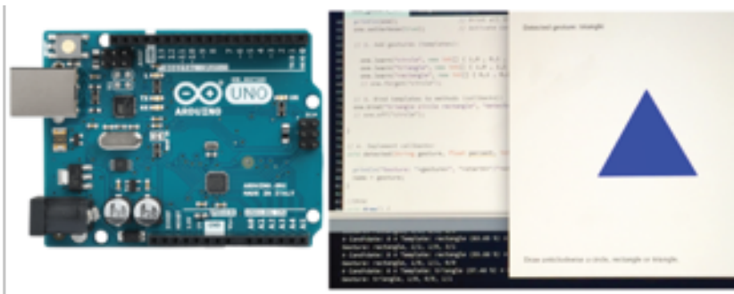
Figure 4.4: Left image of an Arduino Uno, it was used to read the lines of the 8x8 matrix of conductive lines in the Zebra fabric. Right: Processing interface and GUI of test app developed that included the $1 Dollar recognizer and detect gestures, on the image a triangle was detected and draw on the GUI.
