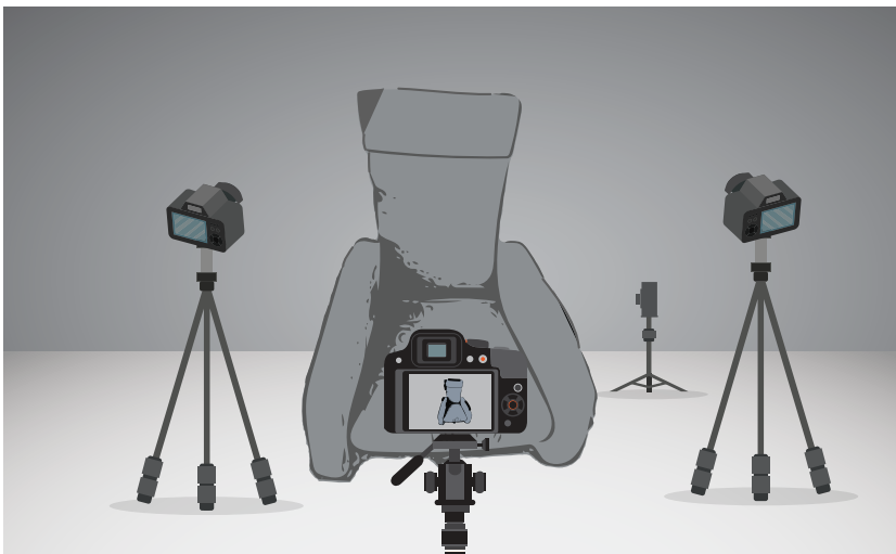
Figure 3.1: Sketch of the evaluation setting performed for the elicitation study. The armchair where each participant is to sit and interact with, surrounded by a set of four cameras: front, left corner, right corner, one on the side of the participant dominant hand.
