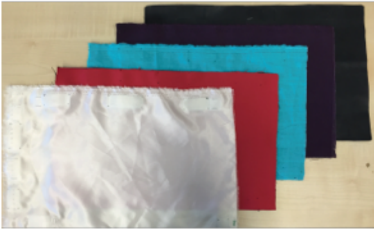
Figure 5.1: View of the 5 fabric texture samples used in the preliminary study. Bottom left to top right view in the following order: white silk, red blackout fabric, blue linen, purple canvas cotton and black leather.
