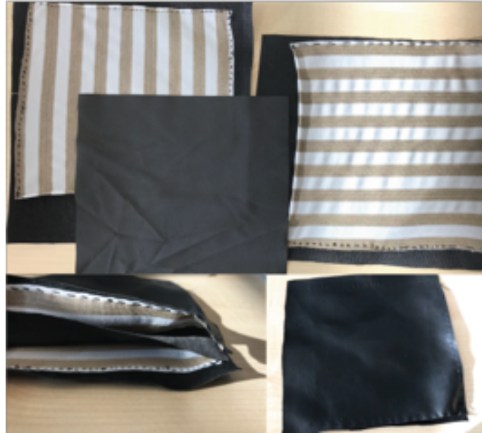
Figure 4.3: Implementation of prototype 4, a resistive pressure touch pad. Top image: layer involved, horizontal position zebra swatch, vertical positioned zebra swatch and piezo resistive fabric. Down left: front view of the pad setup, all layers at view. Down right: top view of the setup.
