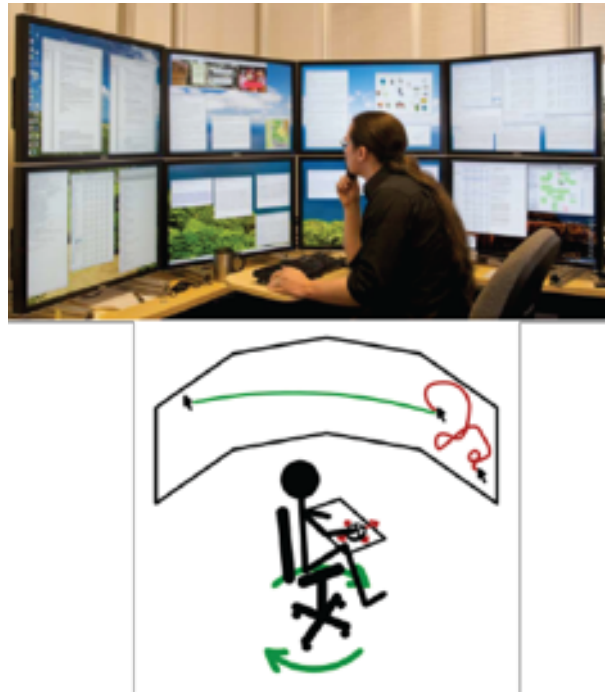
Figure 2.5: Illustration demonstrating how chair rotation would translate to pointer in display Endert et al. [2011]
