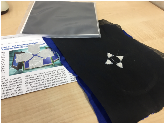
Figure 4.2: Implementation of prototype 3, a pressure sensor with the shape of triangular buttons embroidered in fabric.
