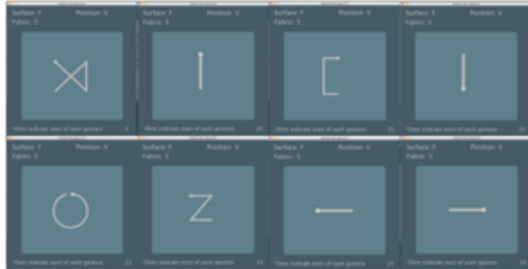
Figure 6.4: Example of a sequence of gestures presented in the test application. From top left to bottom right the sequence is as follows: “X”, swipe down, left bracket, swipe up, circle, “Z”, swipe right and swipe left. Each of this sequences is to be repeated 4 times and the sequences changes each time another independent variable [stiffness of underlying surface, position on chair, texture of fabric] is updated.
