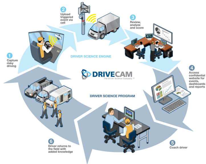
Figure 3.8: DriveCam system feedback loop 1
