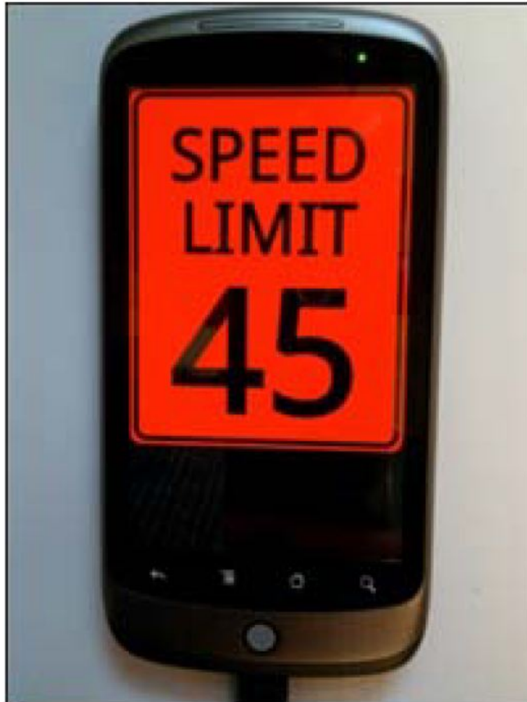
Figure 3.4: Visual feedback when exceeding the current speed limit in the Teen Driver Support System
