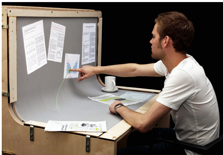
Figure 1.1: BendDesk seamlessly merges a horizontal and a vertical surface into one large interactive surface by a curve.
