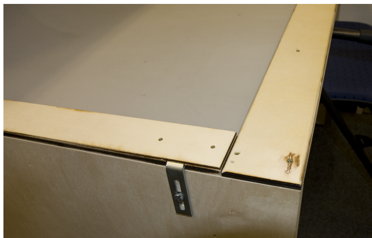
Figure 5.6: Laths on top of the acrylic surface that hold all layers in place.
