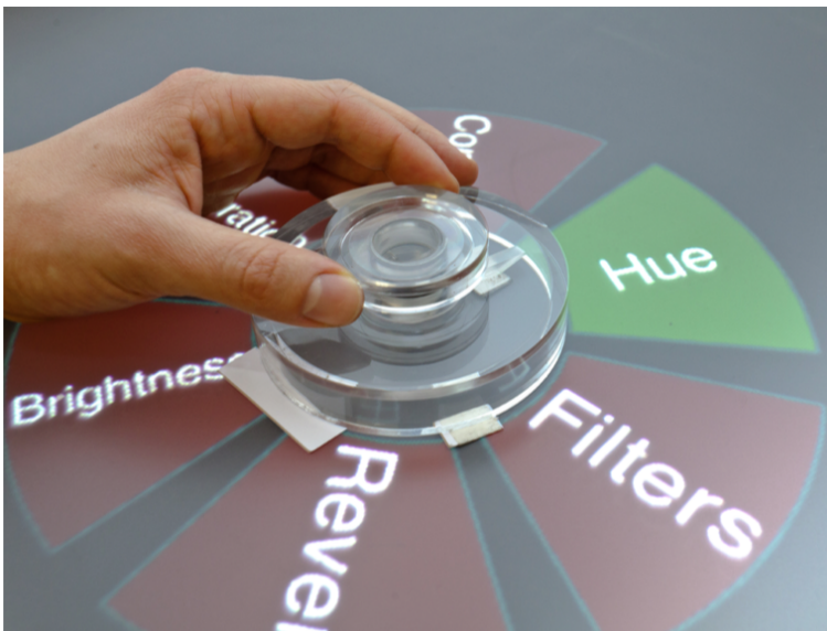
Figure 4.2: SLAP knobs allow controlling digital contents with physical objects. In this example, the SLAP knob is used to change properties of an image displayed on the touch-screen. Image courtesy of Weiss [2012].
