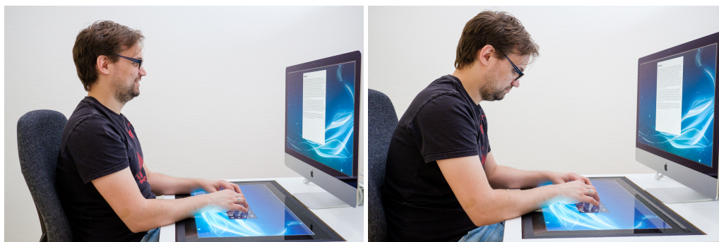
Figure 1.4: Due to the lack of haptic feedback on interactive tabletops, users have to constantly look at their hands to make sure that they interact with the correct digital content. In this example the user cannot “feel” the keys. Therefore, he has to constantly switch his focus between the digital document (left) and the digital keyboard (right).
