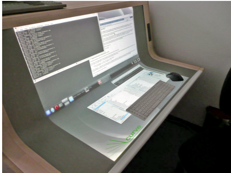
Figure 2.3: The Curve system combines a horizontal and a vertical surface into one large interactive surface. [Wimmer et al., 2010]
