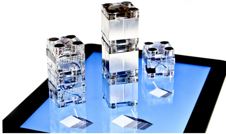
Figure 4.3: Capstone blocks on an iPad allow stacking but are only detected if touched by a user. Image courtesy of Chan et al. [2012]
