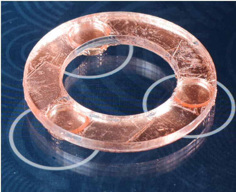
Figure 4.8: With the three pads we ensure that at least one area of the marker is always capacitively coupled with several inactive intersections, independent of its orientation.
