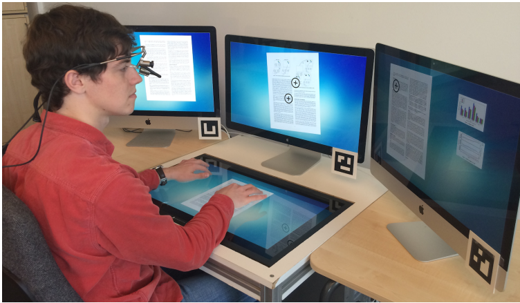
Figure 5.1: Concept of how our gaze supported interaction-techniques can be applied to multi-screen desk workspaces. In this setup users are able to interact with multiple vertical screens while creating the input on the horizontal surface [Voelker et al., 2015b].
