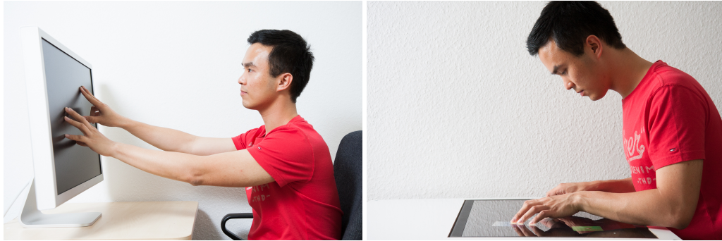
Figure 1.3: The issues of vertical and horizontal touch-screens: Left: Directly interacting with the vertical screen is cumbersome and leads to the gorilla arm effect [Hincapié-Ramos et al., 2014]; Right: Constantly looking at the horizontal surface leads to neck pain [Bachynskyi et al., 2015].
