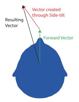
**Figure 5.8:** The forward-vector was used as direction-vector. If the angle  $\alpha$  exceeded a threshold, the vector created through side-tilt was added to the direction-vector.
