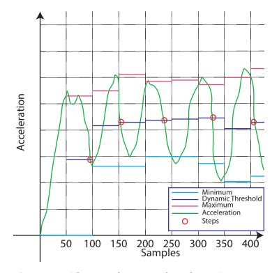
**Figure 5.7:** The step-detection algorithm. A step event is triggered, when the acceleration falls below a dynamic threshold. This threshold is adjusted every 50 samples.
