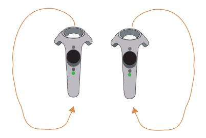
**Figure 2.2:** Arm-cycling is a breast-stroke like armmovement. The displacement of the controller is used to control velocity
