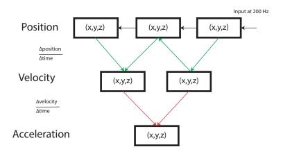
**Figure 5.6:** The deriving of acceleration out of positional data. The data is sampled into a ring buffer. On every new sample the positions are derived into velocity and then into acceleration.
