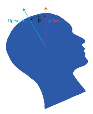
**Figure 5.10:** The angle  $\beta$  is the angle between the up-vector of the users head and the y-axis calculated from the side.
