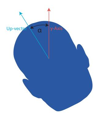
**Figure 5.9:** The angle  $\alpha$  is the angle between the up-vector of the users head and the y-axis calculated from the front.
