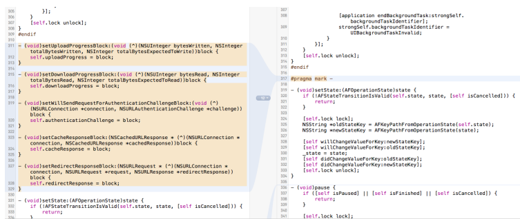
Figure 1.7: File comparison view in Apple’s Xcode. The difference annotations easily show how the five methods on the left were deleted sometime between the two versions. Interestingly, this display is incorrect. The methods were actually moved somewhere else in the file, but the Diff algorithm chosen by Xcode could only model this as a delete here and an insert at the new location.
