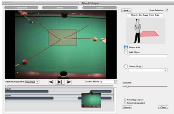
Figure 2.11: The timeline interface to highlight time ranges of object movement patterns. Here we see that the selected objects, the red and the yellow ball, will enter and leave the orange region simultaneously.
