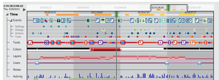
Figure 2.1: Stacked timeline visualization with editing events. The hierarchical nature of the annotations allows to summarize individual event timelines in a group and allows to hide unwanted details. From [Grossman et al., 2010]
