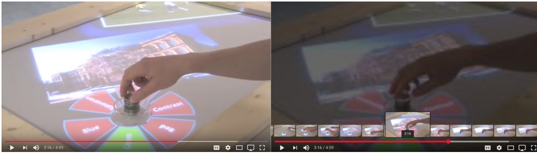
Figure 1.2: The Youtube playback interface with a typical timeline slider at the bottom. The interface on the right shows frames surrounding the current playhead. These provide additional context and help the user to find navigation targets.
