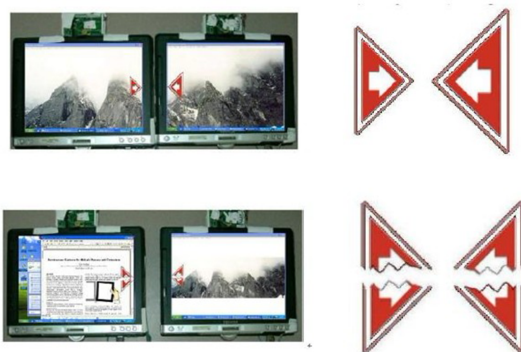
Figure 4.20: visual feedbacks for the dynamic display tiling, which indicate the connection and disconnection of the displays. Top left and right: the device on the left side bumps into the one on the right side, the arrow with larger size indicates the connecting display. Down left and right, these two splitting arrows indicate that one tablet is moved away from the other one and the connection is broken.
