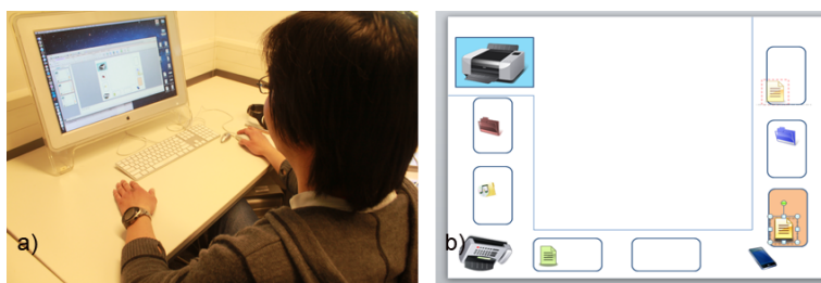
Figure 5.5: Applying the prototype of Radar View : a) a user is dragging a file icon to another computer on the map; b) the screenshot of the map.
