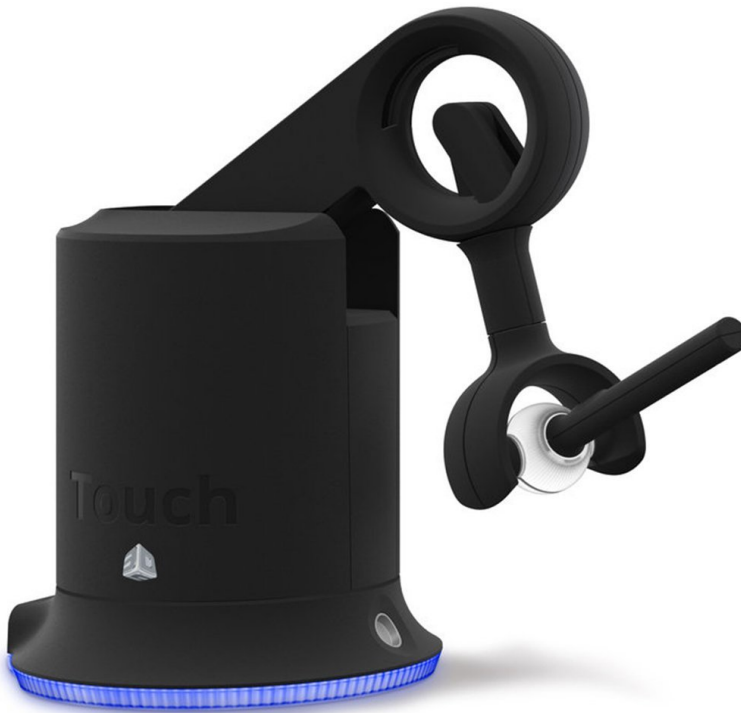
Figure 3.1: The Touch 3D stylus from 3D Systems is a 6 DoF haptic device. It comes with the SDK OpenHaptics to control the force input on the handle motors.
